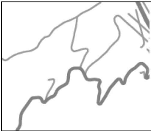
Many dead-ends and 3-way intersections are indicators of poor connectivity.
