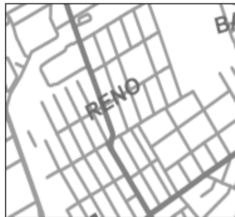
Many 4-way intersections are indicators of good connectivity.
