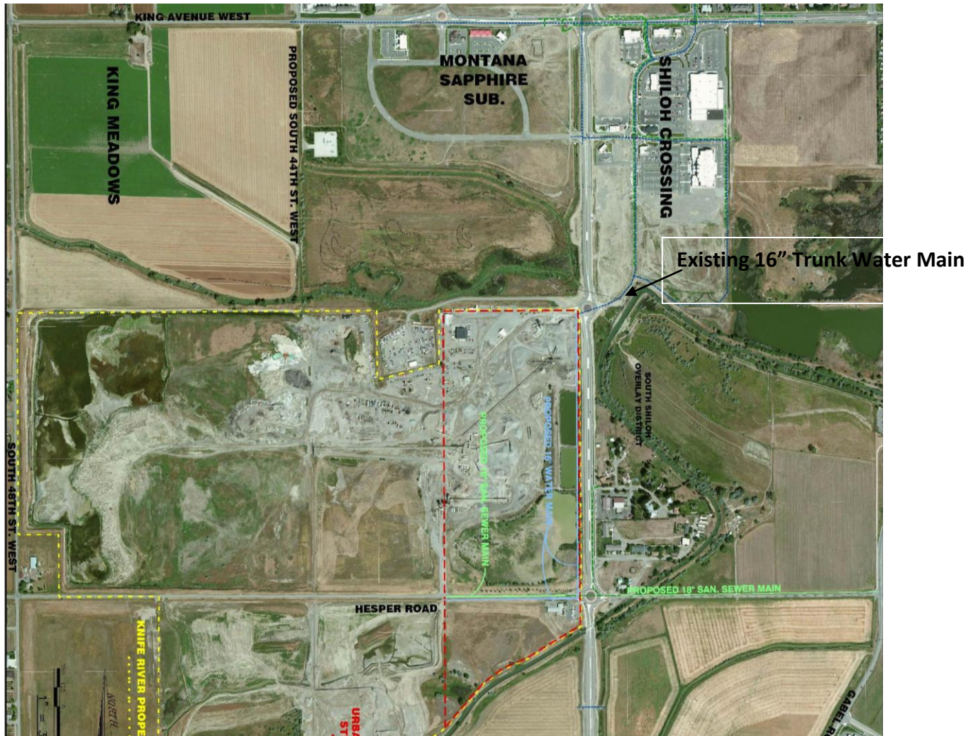
Figure 4: Existing and Proposed Water and Sewer
