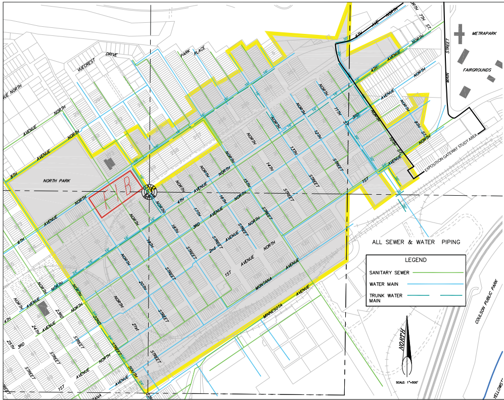
FIGURE 2-5 EBURD SEWER AND WATER PIPING
