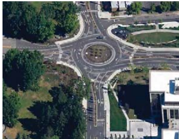
FIGURE 2-19 MAJOR INTERSECTION ROUNDABOUT
