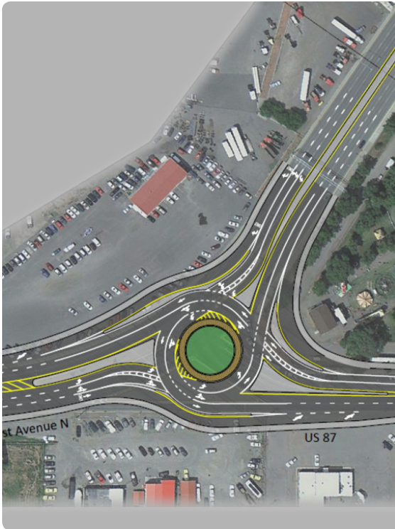
Figure 2.02 – Long-term recommendations for the corridor include a “signature” roundabout at 1st Avenue/US 87. Such a feature would address multiple goals for the corridor, but would require coordination and funding from MDT and other agencies. (Image source: Fehr & Peers, Sanderson-Stewart)
