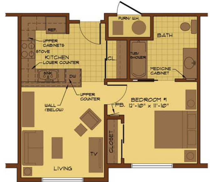
3 SINGLE UNIT BLOW-UP (STANDARD) 1 BED. APARTMENT QTY 9 SCALE: 1/4"=1'-0" AREA = 582 SF.
