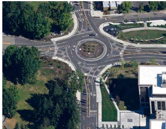
FIGURE 2-19 MAJOR INTERSECTION ROUNDABOUT
