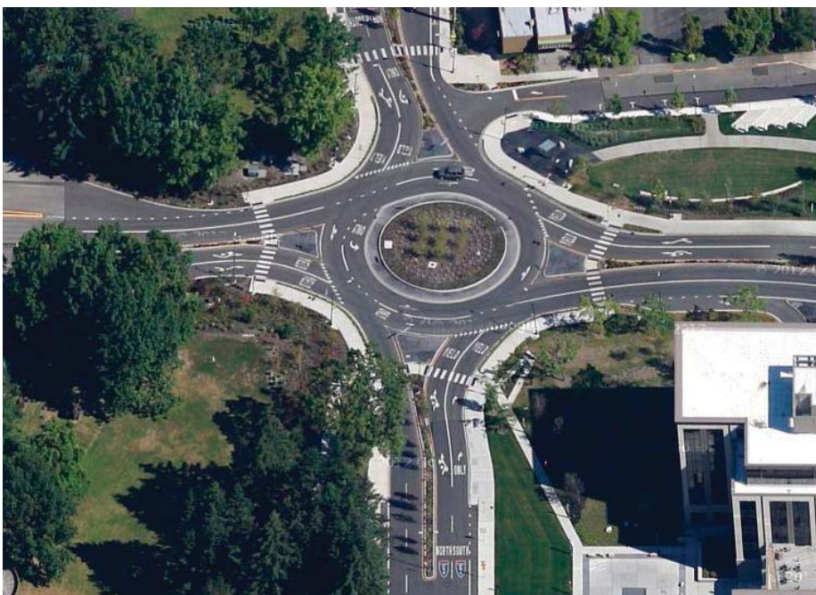
FIGURE 3-6 EXAMPLE OF ROUNDABOUT CONNECTION TO THE INTERSTATE
