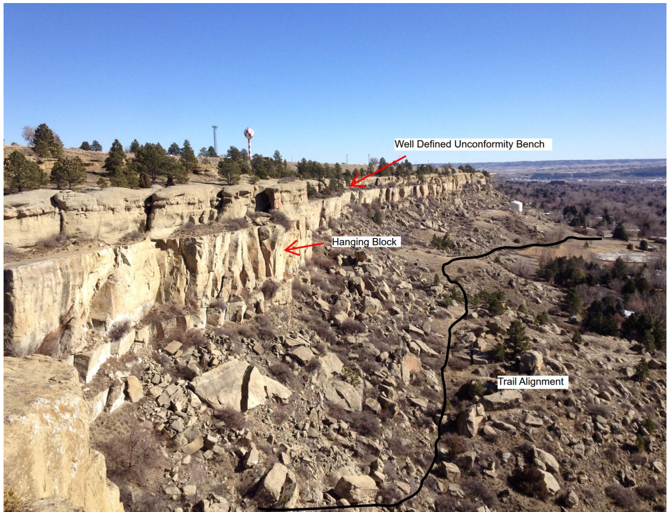
Looking east toward 17 th Street. Note the east half of the alignment follows along a landslide bench that appears outside of the modern run-out zone. The west half of the alignment appears at the bottom of the modern run-out zone.
