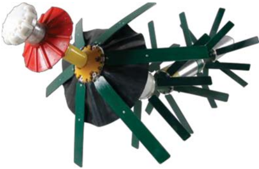
Figure 3: PipeDiver Free-swimming Electromagnetic Inspection Tool
