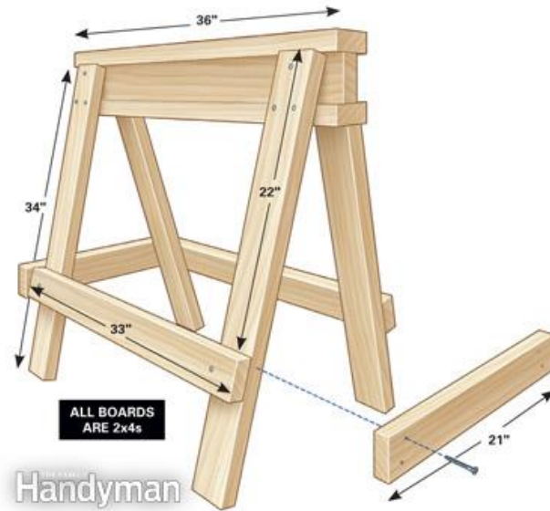
Figure I-3i: Suggested design for sawhorse legs
