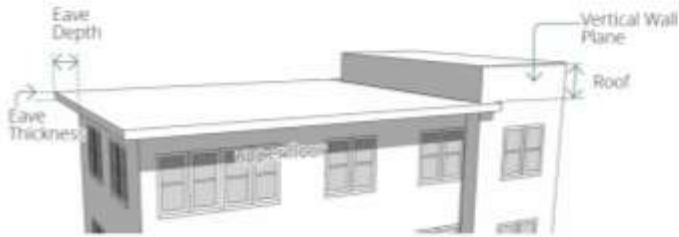
Example of a Flat Roof
