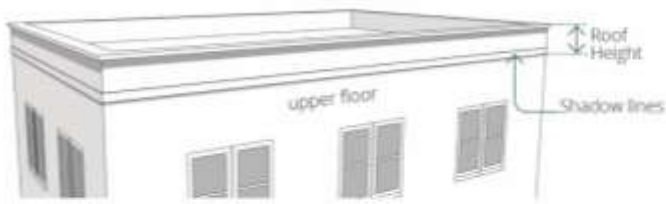
Example of a Parapet e
