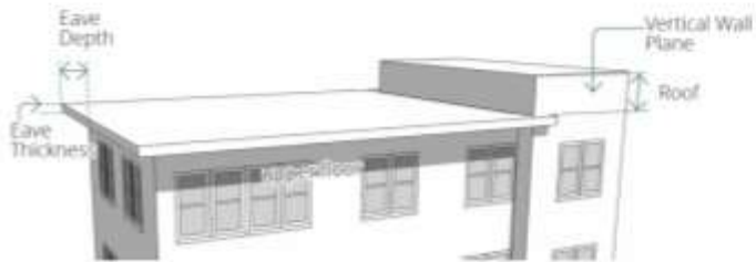
Example of a Flat Roof
