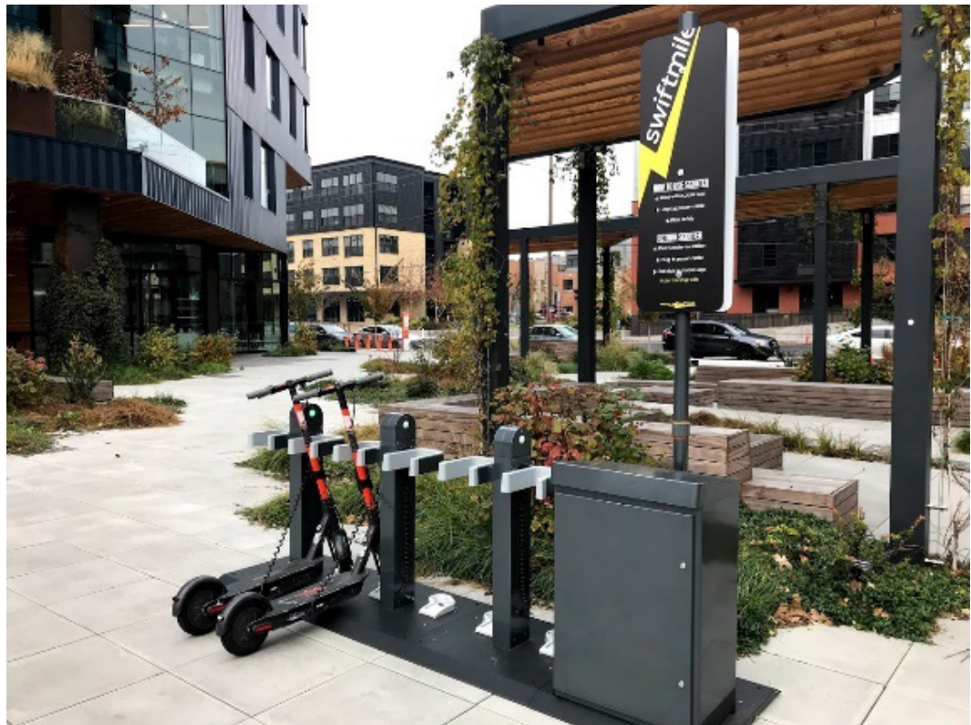
An electric charging hub with docks for scooters.
