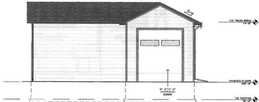
NORTH ELEVATION SCALE: 1/4" = 1'-0"
