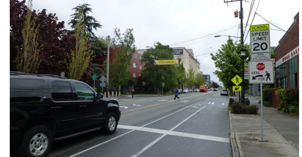
Advanced stop bars increase visibility of people crossing the street
