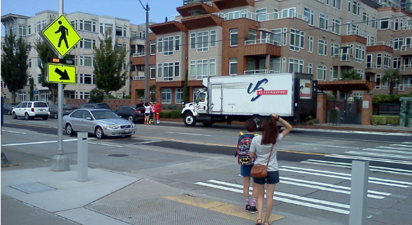
RRFB with passive detection
