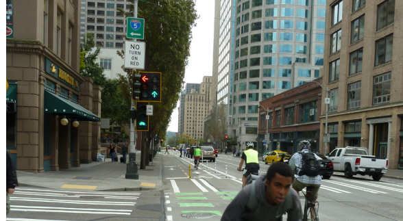
Reflective back plate makes the signal more visible
