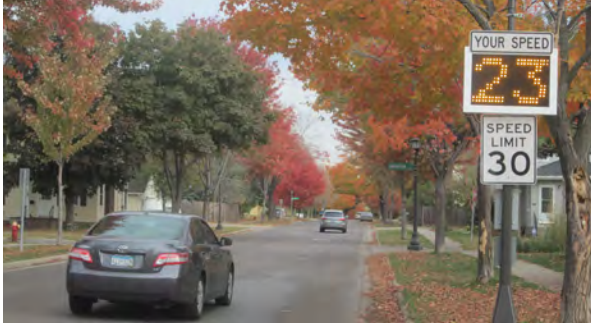
Speed feedback sign displays a driver's speed compared to the speed limit
