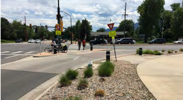
Slip lanes with added signs and raised crosswalks bring attention to pedestrians
