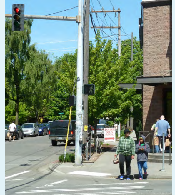
With a Leading Pedestrian Interval, motorists have a red signal for the first 3–5 seconds of the WALK phase.
