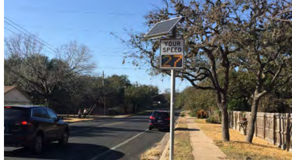
Solar-powered speed radar sign
