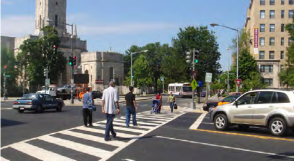
Marked crosswalk at an intersection
