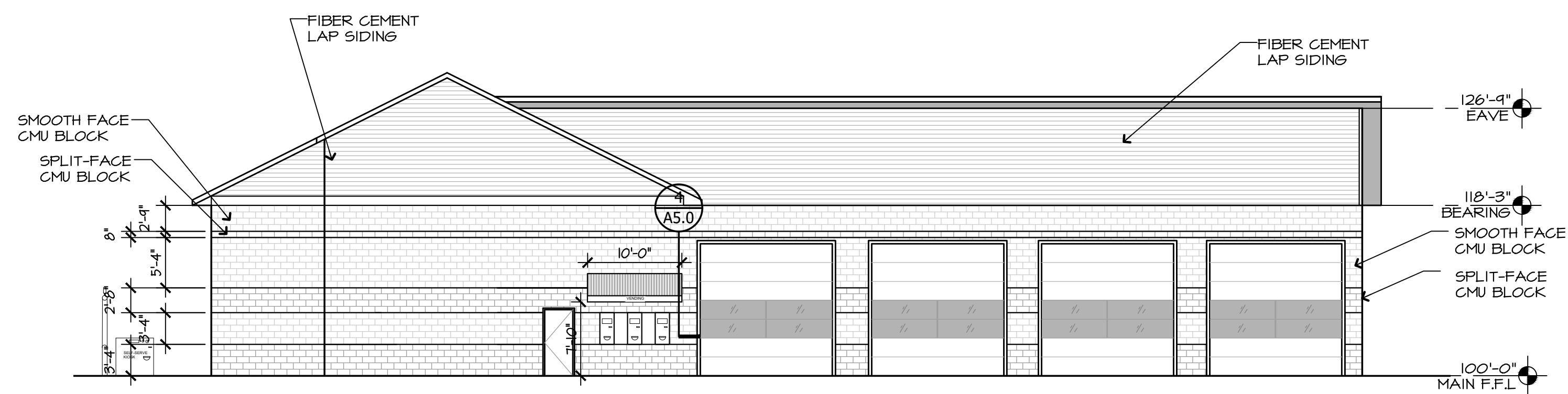
4 RIGHT ELEVATION Scale: 3/32" = 1'-0"
