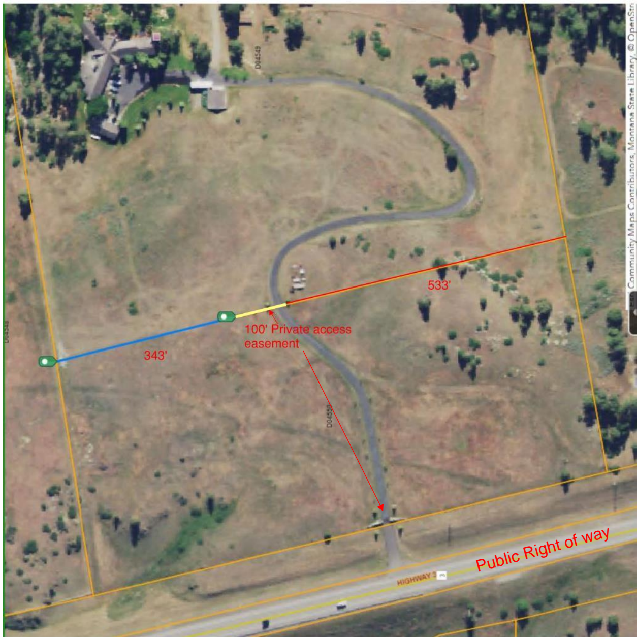
Aerial photo view of approximate edge of access easement (measurements). (not part of easement document) (Not part of zoning code)
