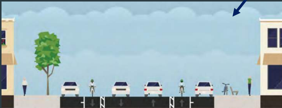
8 | 6.5 | 10.5 Lanes | 6.5 | 8 Buffered Bike Lane - Division to N 31st St; N 25th St to N 22nd St
