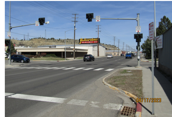
Pedestrian Hybrid Beacon (PHB). Source: DOWL
