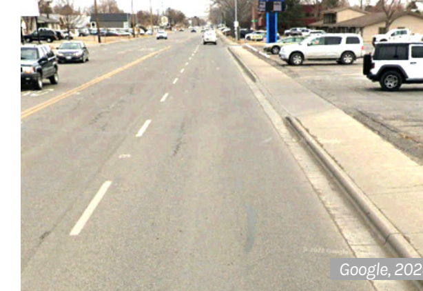
This sidewalk on Broadwater Ave. has some protection because of the curb, but is not separated. This is called “curbwalk” and should be avoided as an SRTS solution whenever possible.
