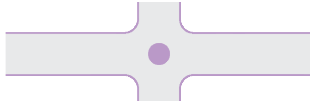
Figure 2.01 - Traffic Circles Traffic Circles reduce traffic speeds at intersections by requiring motorists to move with caution through conflict points.
