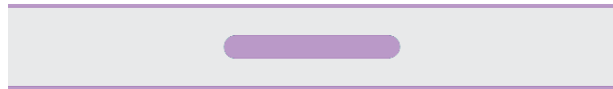
Figure 2.01 - Median: Medians create a pinch-point for traffic in the center of the roadway and, when they include pedestrian refuge islands, can reduce crossing distances
