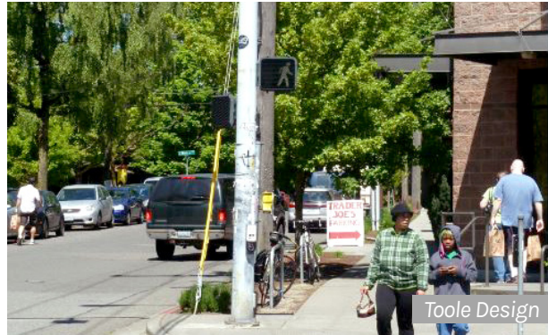
With a Leading Pedestrian Interval, motorists have a red signal for the first 3–5 seconds of the WALK phase
