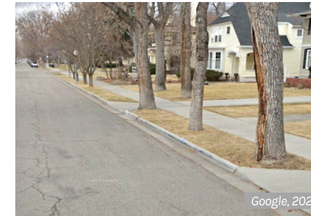
This sidewalk on Clark Ave. is separated and, because of the curb and frequent street trees, has a higher level of protection.
