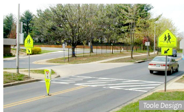
In road signage reinforces pedestrian priority at school crossings
