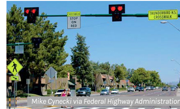
A PHB in Phoenix, AZ provides added visibility for pedestrians near a high school
