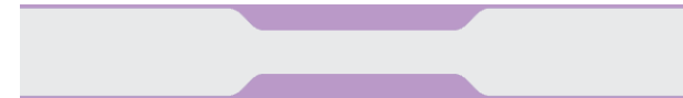
Figure 2.02 - Pinch-point: Pinch-points restrict vehicles from moving at high speeds and can expand the sidewalk for pedestrians at intersections as curb extensions or at mid-block locations.
