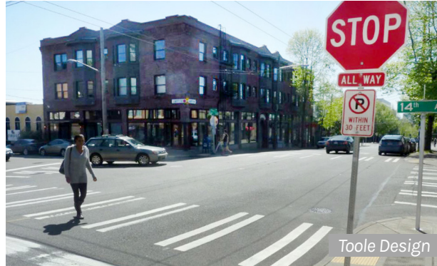
Stop sign with stop line at an all-way stop
