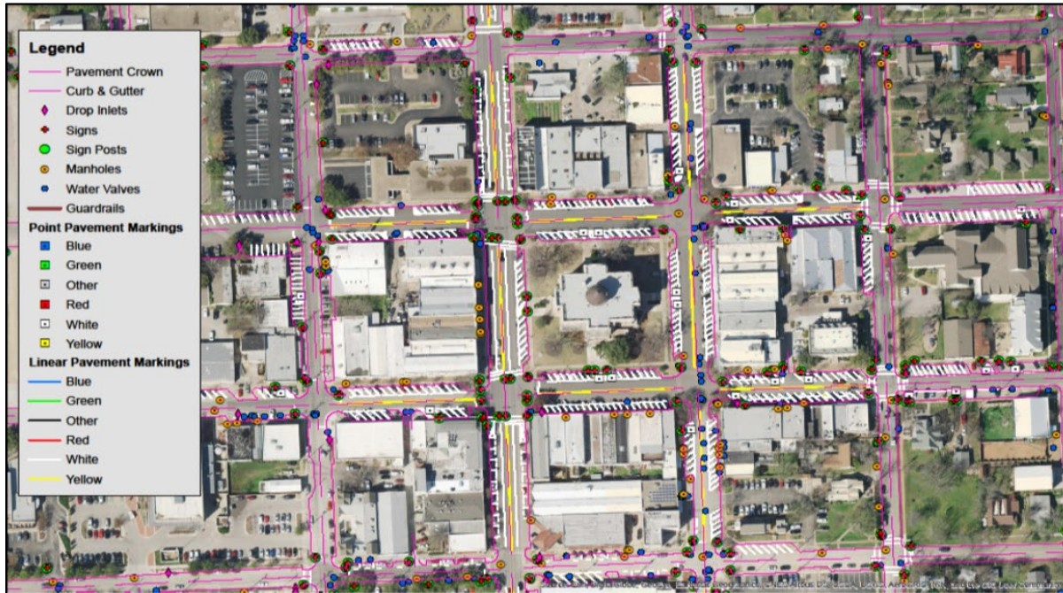
Figure 3.4 GIS-Based Asset Inventory Deliverables
