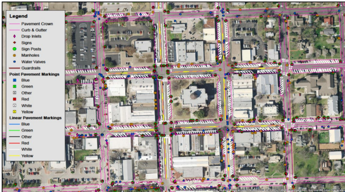
Figure 3.4 GIS-Based Asset Inventory Deliverables
