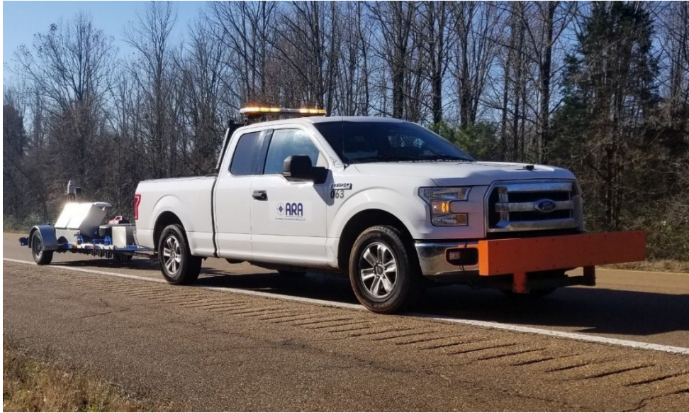
Figure 3.5 ARA's Falling Weight Deflectometer.
