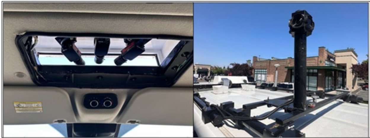
Figure 3.1 Right-of-Way HD Cameras and 360° Ladybug Camera
