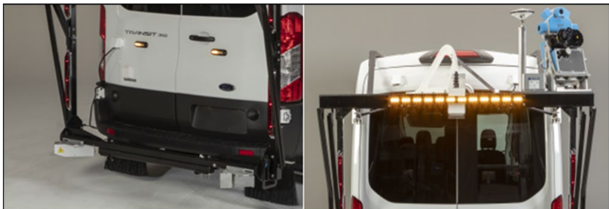
Figure 2.3 PathRunner Profiler and 3D PAS Sensor
