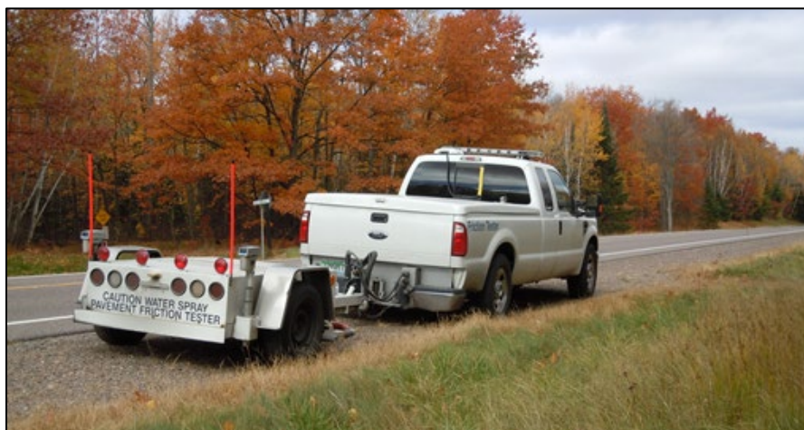
Figure 3.7 ARA's Friction Testing Unit.
