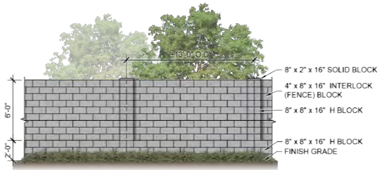
7 6'-0" DOOLEY WALL ON 2'-0" MAX. RETAINING WALL
