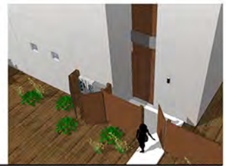
SES elec panel enclosure incorporated into the private yard fencing
