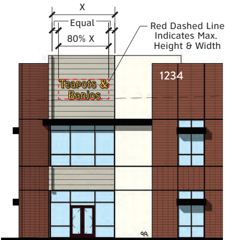
SINGLE TENANT ENTRY SIGN PLACEMENT - TYP. Scale: 1/16"=1'-0"
