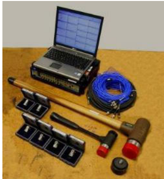
Figure 2. Typical equipment needed for Operating Deflection Shape (ODS) testing and experimental modal analysis (impact testing) includes: the laptop computer with the data analysis software installed, analyzer with appropriate channel count, associated cables, the required number of above tri-axial accelerometers and uni-axial accelerometers, and an instrumented impact hammer.
