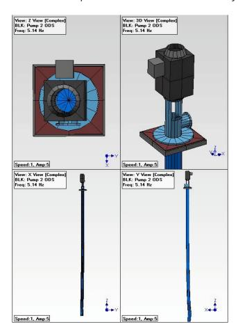
**Figure 4.** Static image of an ODS animation of a vertical pump system. ODS animation overlay test data on an MSI prepared 3D solid model. When animated looseness, deflections, and natural frequencies can be viewed to identify problems with more certain so a fix can be recommended with more confidence.
