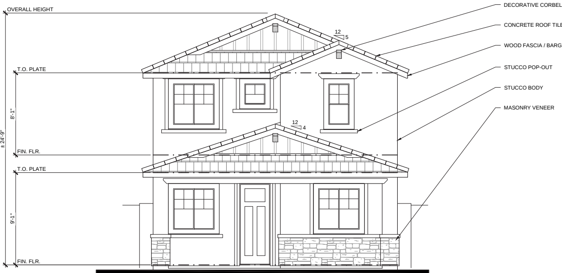
FRONT ELEVATION ELEVATION B - FARMHOUSE 1/4" = 1'-0"
