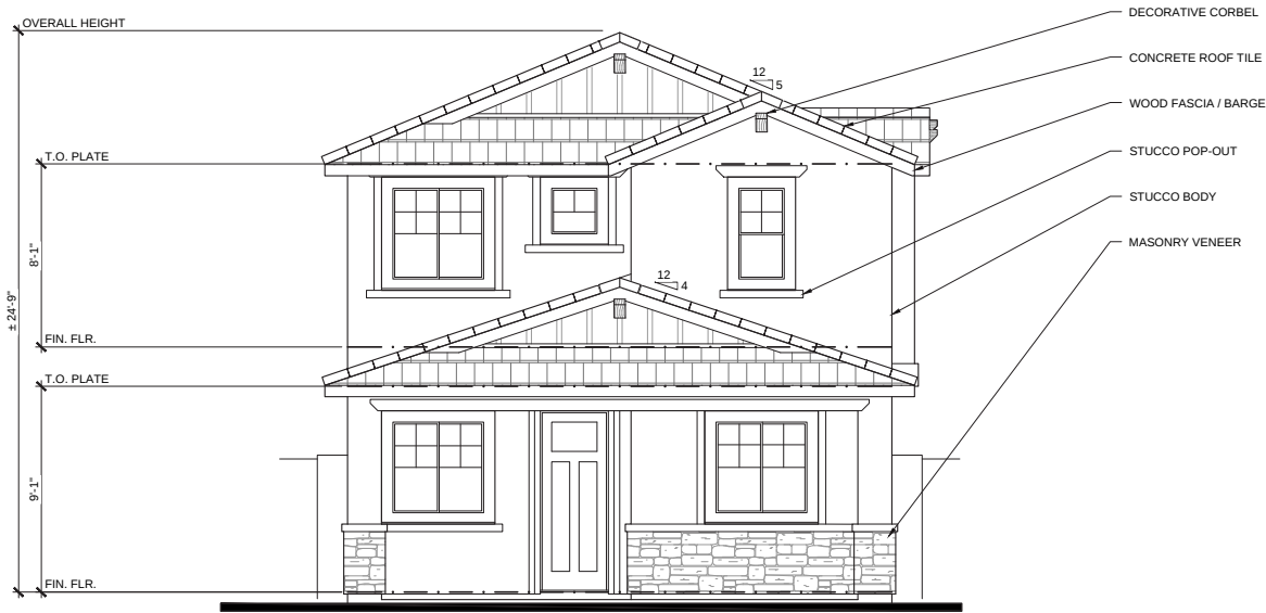
ENHANCED LOT FRONT ELEVATION ELEVATION B - FARMHOUSE 1/4" = 1'-0"
