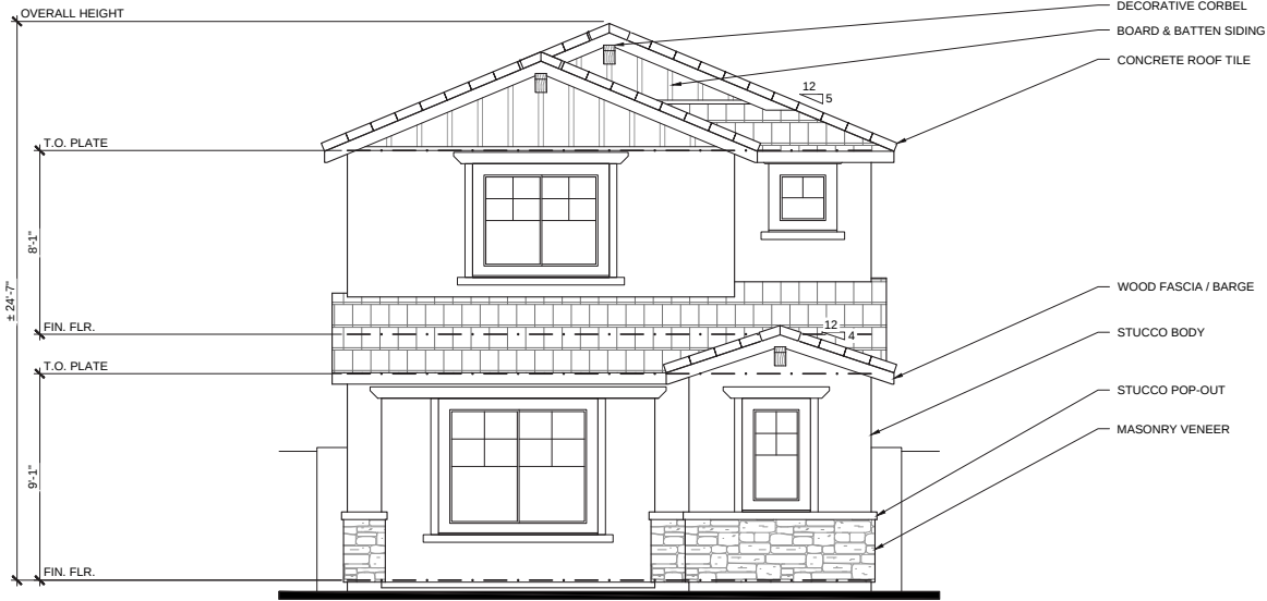
FRONT ELEVATION ELEVATION B - FARMHOUSE 1/4" = 1'-0"
