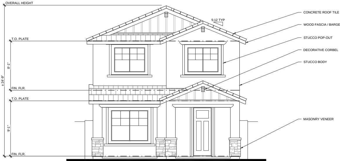
FRONT ELEVATION ELEVATION B - FARMHOUSE 1/4" = 1'-0"
