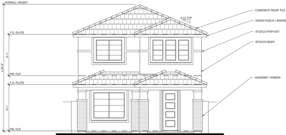
FRONT ELEVATION ELEVATION C - DESERT MODERN 1/4" = 1'-0"
