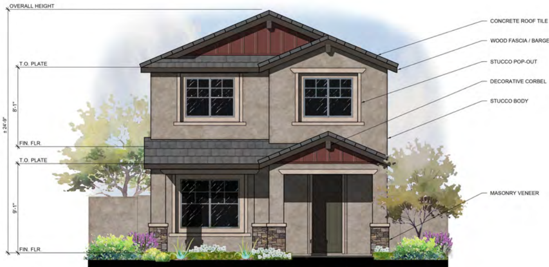
FRONT ELEVATION ELEVATION B - FARMHOUSE 1/4" = 1'-0"
