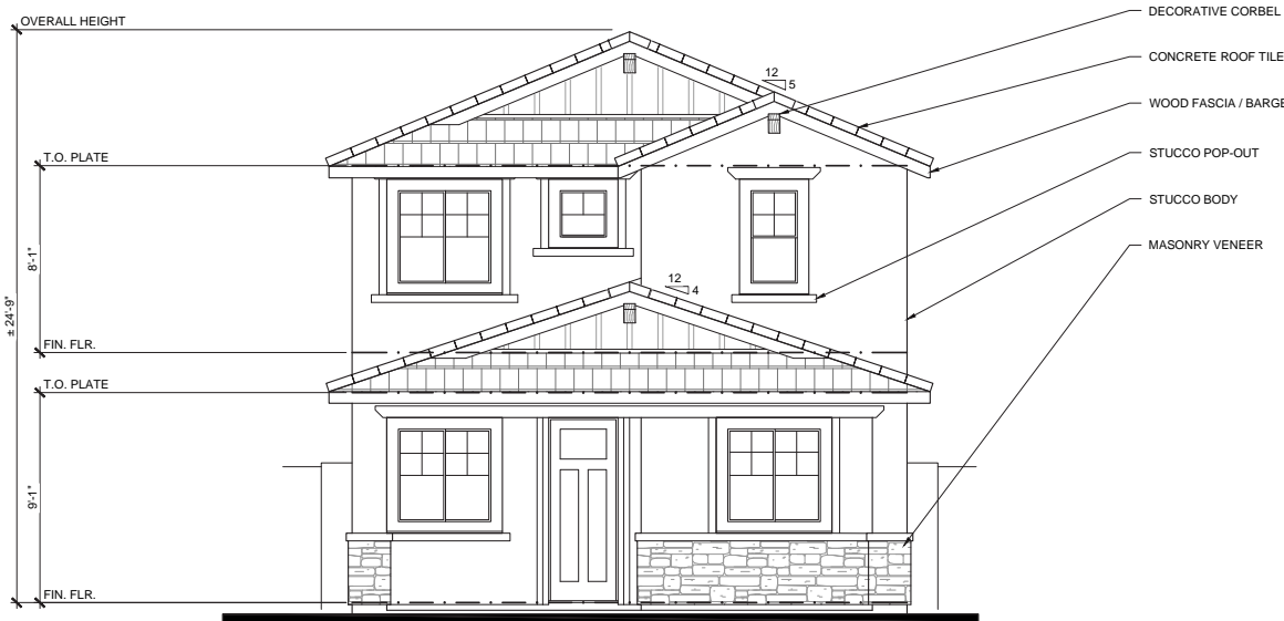
FRONT ELEVATION ELEVATION B - FARMHOUSE 1/4" = 1'-0"
