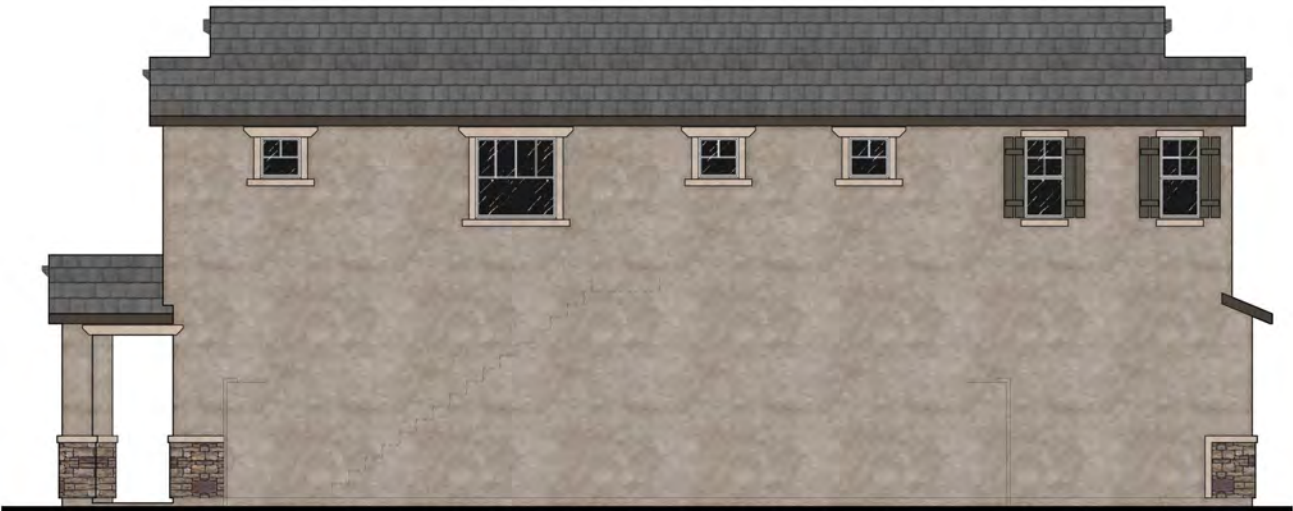
RIGHT ELEVATION ELEVATION B - FARMHOUSE 1/4" = 1'-0"
