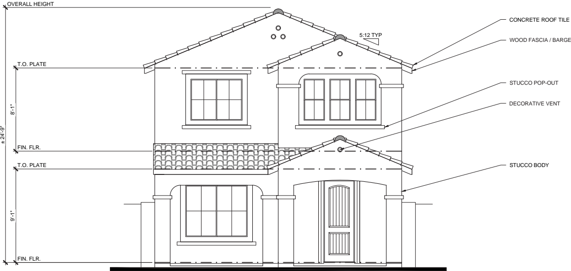
FRONT ELEVATION ELEVATION A - SPANISH 1/4" = 1'-0"
