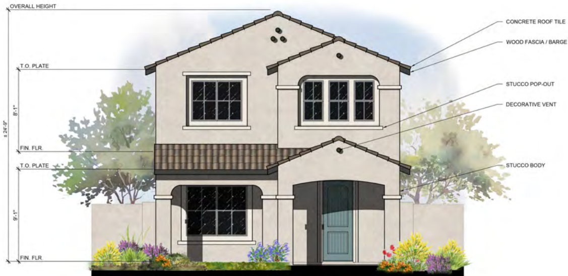
FRONT ELEVATION ELEVATION A - SPANISH 1/4" = 1'-0"
