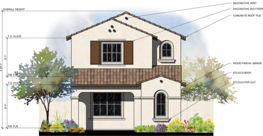
FRONT ELEVATION ELEVATION A - SPANISH 1/4" = 1'-0"
