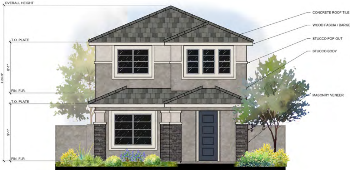
FRONT ELEVATION ELEVATION C - DESERT MODERN 1/4" = 1'-0"
