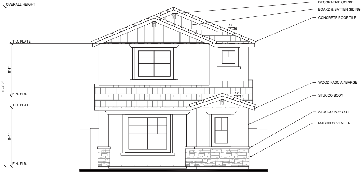
FRONT ELEVATION ELEVATION B - FARMHOUSE 1/4" = 1'-0"
