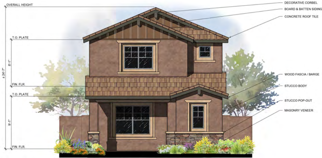
FRONT ELEVATION ELEVATION B - FARMHOUSE 1/4" = 1'-0"
