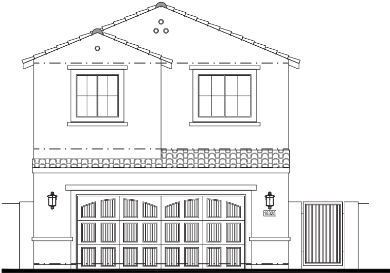
REAR ELEVATION ELEVATION A - SPANISH 1/4" = 1'-0"
