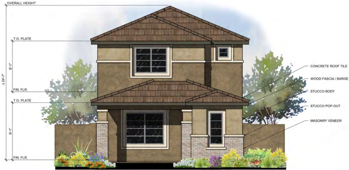
FRONT ELEVATION ELEVATION C - DESERT MODERN 1/4" = 1'-0"
