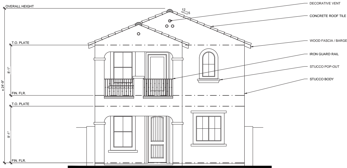
FRONT ELEVATION ELEVATION A - SPANISH 1/4" = 1'-0"
