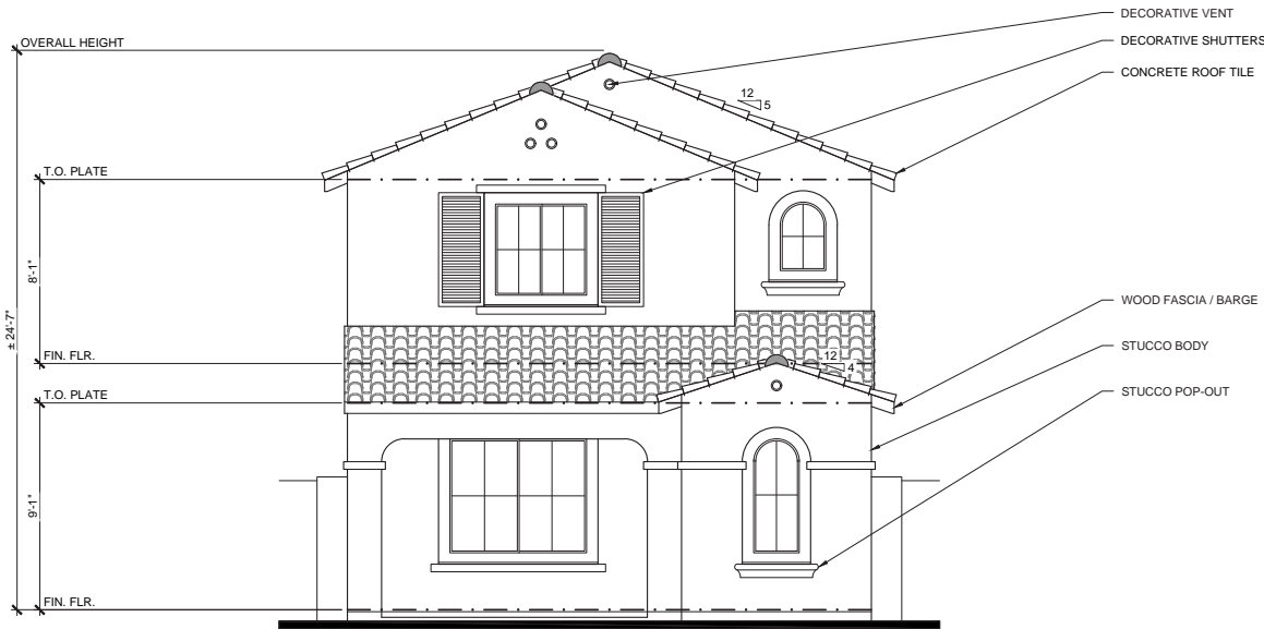
FRONT ELEVATION ELEVATION A - SPANISH 1/4" = 1'-0"
