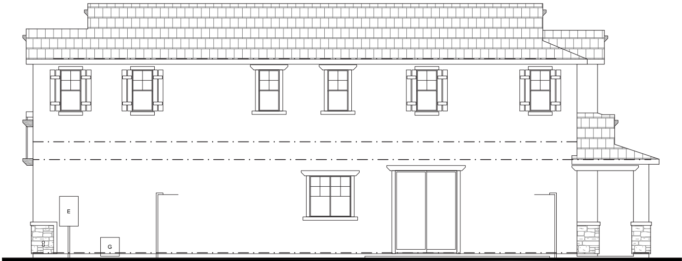
LEFT ELEVATION ELEVATION B - FARMHOUSE 1/4" = 1'-0"
