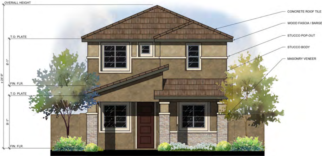
FRONT ELEVATION ELEVATION C - DESERT MODERN 1/4" = 1'-0"
