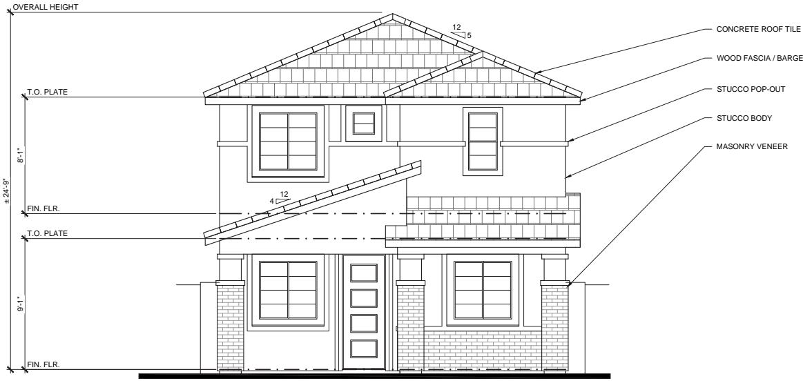
FRONT ELEVATION ELEVATION C - DESERT MODERN 1/4" = 1'-0"
