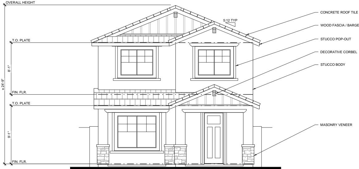
FRONT ELEVATION ELEVATION B - FARMHOUSE 1/4" = 1'-0"
