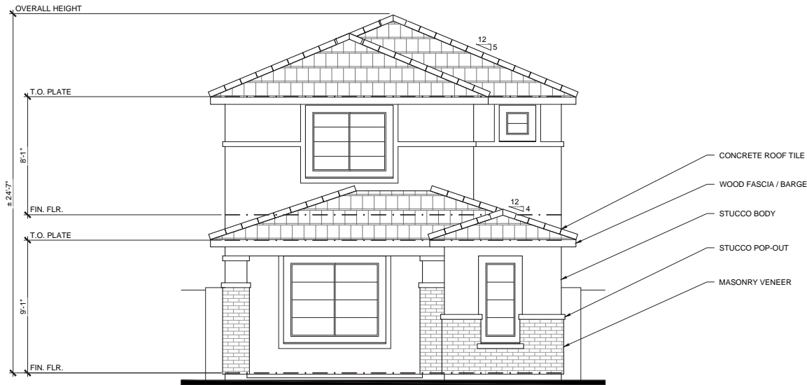
FRONT ELEVATION ELEVATION C - DESERT MODERN 1/4" = 1'-0"
