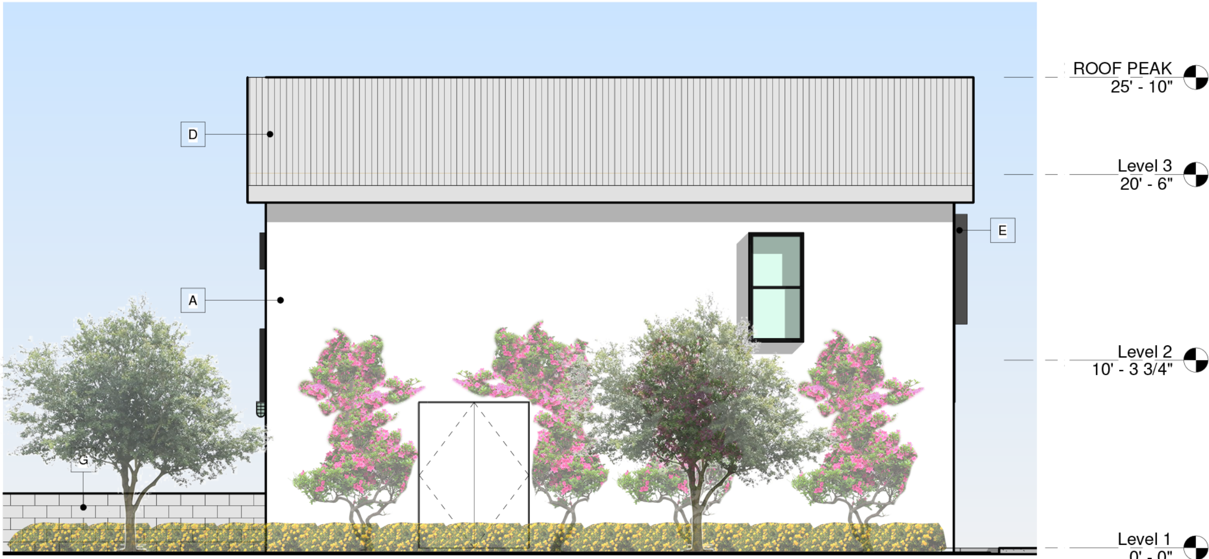
4 SOUTH ELEVATION (FRONT UNITS) 3/16" = 1'-0"
