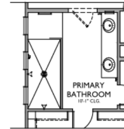
FRAMELESS WALK-IN SHOWER AT PRIMARY BATHROOM
