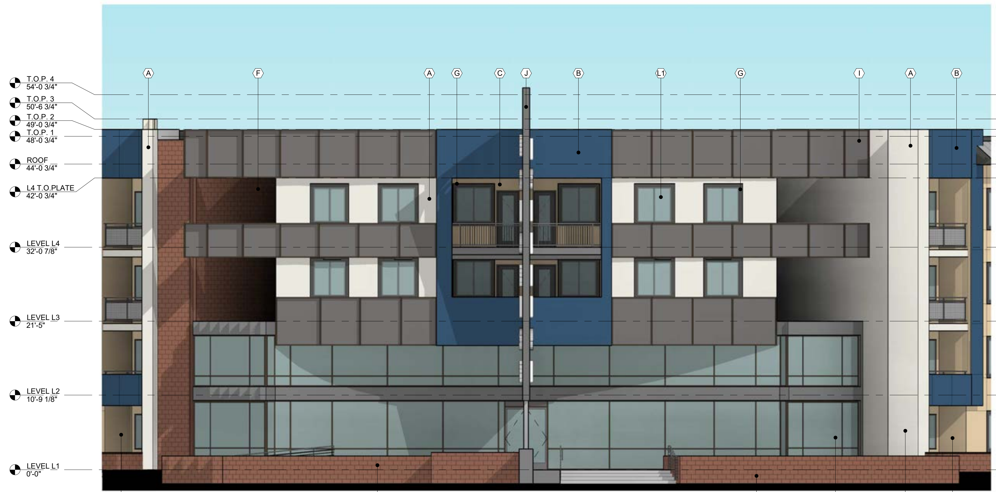
2 ENLARGED LEASING ENTRY ELEVATION SOUTH EAST SCALE: 1/8" = 1'-0"
