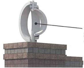
LOGO TO BE MADE OUT OF ALUMINUM AND STUD MOUNTED ON WALL TO MAKE 3-DIMENSIONAL GRAPHIC. FINAL COLORS TBD.
