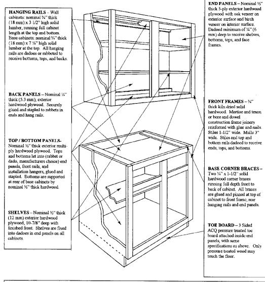
**DRAWERS** – 11/16" thick solid pine lumber four sided drawer box. Ends are captured in drawer side dadoes. Drawer bottoms are nominal ¼" thick (5.2 mm) hardwood plywood dadoed into all four drawer box sides. All drawer parts are glued and nailed together.
