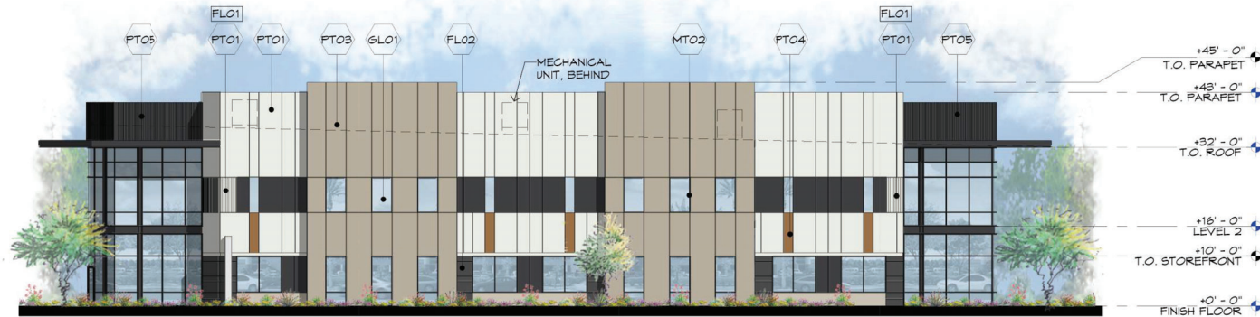
2 BUILDING C - NORTH ELEVATION SCALE: 1/16" = 1'-0"
