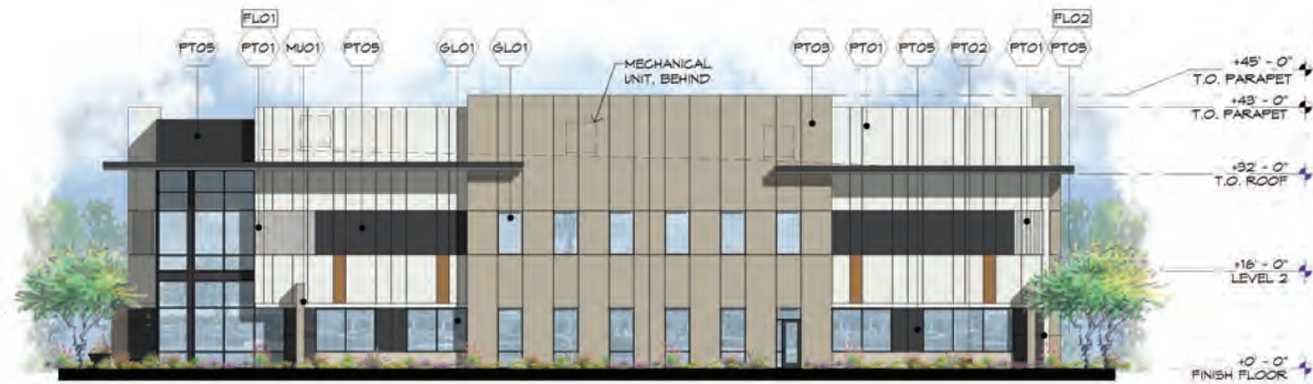
2 BLDG E - NORTH ELEVATION SCALE: 1/16" = 1'-0"
