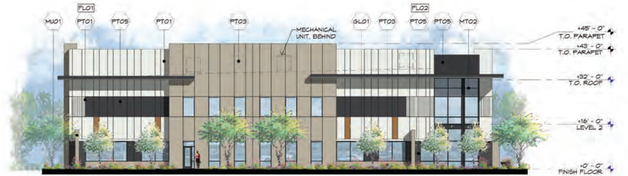
3 BLDG E - SOUTH ELEVATION SCALE: 1/16" = 1'-0"
