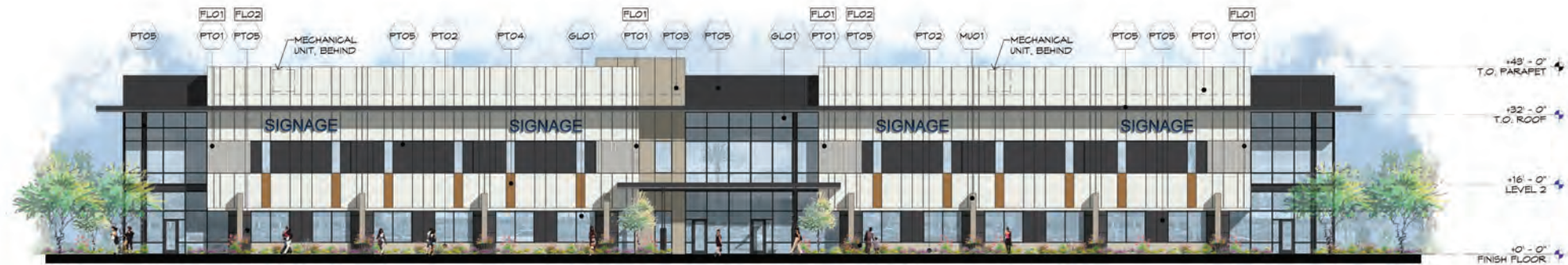
1 BLDG F - EAST ELEVATION SCALE: 1/16" = 1'-0"
