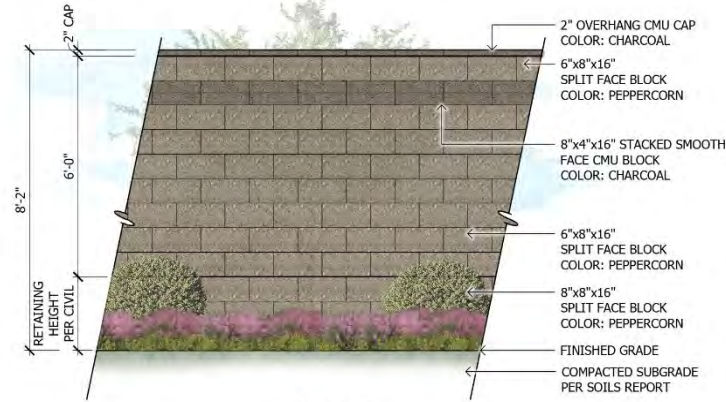
6 Primary Theme Wall on Top of Retaining Wall SCALE: 1/2"=1'-0"
