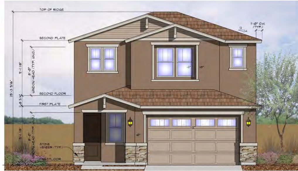
1 FRONT ELEVATION B SCALE: 1/4" = 1'-0"
