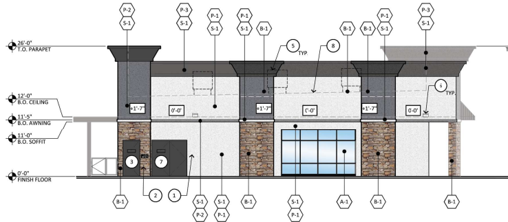
2 EAST ELEVATION - SHOPS BUILDING SCALE: 1/8" = 1'-0"
