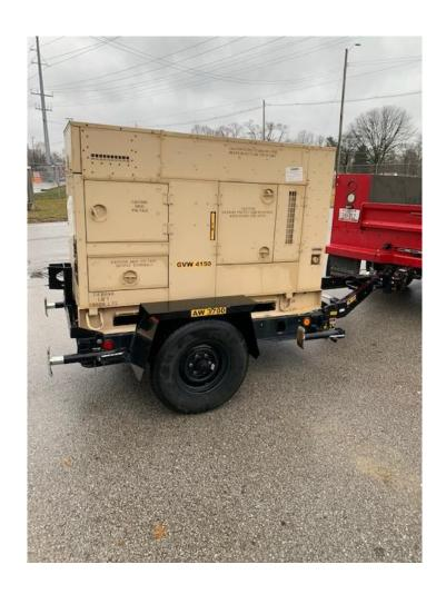
30 KW Diesel Generator Trailer
