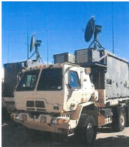
LMTV with UGCS shelter and TDGT 28 ft long x 7 ft wide x 13 ft tall
