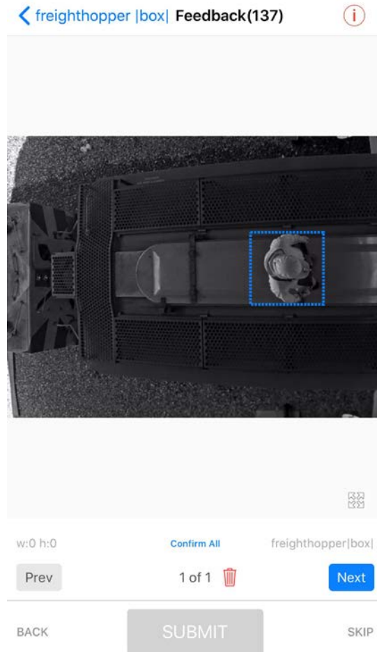
Figure 4 - Application Feedback -- (Mobile). A domain expert can quickly provide confirmation or corrections of Cogniac application predictions.
