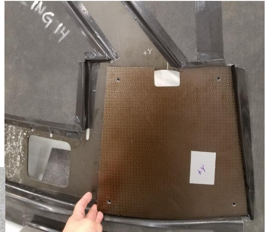
Forward Heat Shield Door 10X12 in./1 lb.
